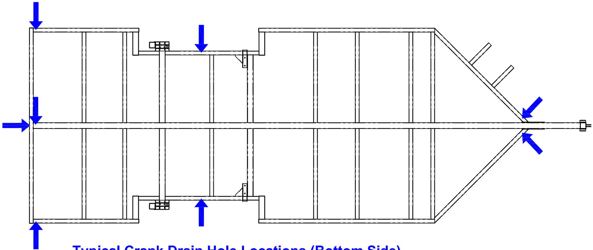
**Typical Crank Drain Hole Locations (Bottom Side)**
